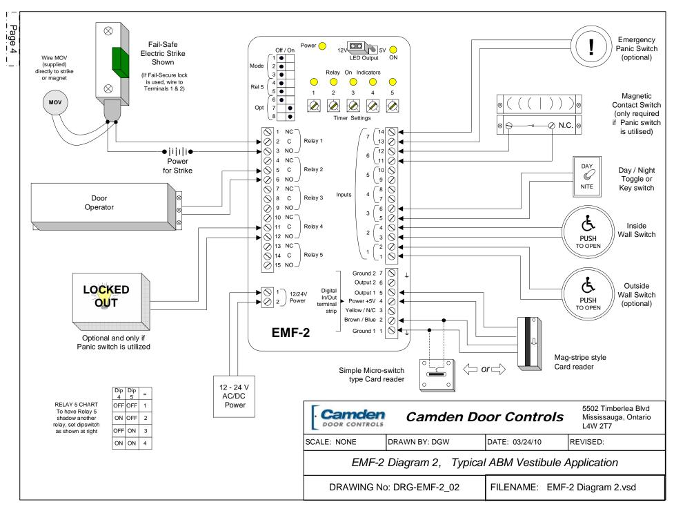
Turn the Key switch (or other type switch) to "Day Mode". If the strike is to be dogged back mechanically, then do so. If it is to be powered all day long, then confirm that it is powered and released.
